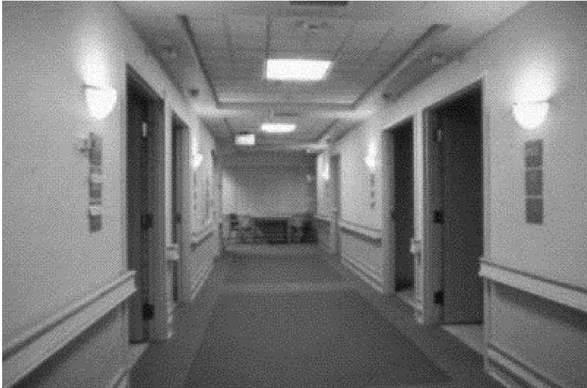
Figure 6-1—Patient corridor, striving for residential feeling (note window treatment at end of corridor and nonglare floor covering)
